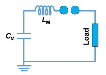
$$I_0 = \frac{V_0}{\sqrt{L_M/C_M}} \quad \omega_0 = \frac{1}{\sqrt{L_M C_M}}$$
