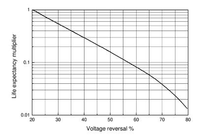
If charge has been injected from the metallic-cathode side into the dielectric, the space charge field associated with it can add to the external field during voltage reversal and the total field can exceed the local breakdown stress and cause damage to the material.
