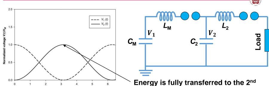
$$V_1 = V_M - \frac{V_M C_2}{C_M + C_2} [1 - \cos(\omega t)] \approx V_M - \frac{V_M}{2} [1 - \cos(\omega t)]$$
