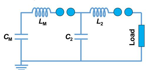
$$I_2 = \frac{V_0}{\sqrt{L_2/C_2}} \qquad \omega_2 = \frac{1}{\sqrt{L_2C_2}}$$
