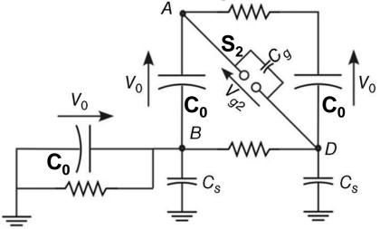
C<sub>s</sub>: between the stage capacitors and ground.
