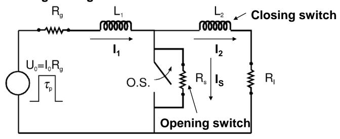
$$R_{g}I_{1} + L_{1}\frac{dI_{1}}{dt} + R_{S}(I_{1} - I_{2}) = 0 \qquad \tau_{\pm} = \left(\frac{R_{l} + R_{S}}{2L_{S}} + \frac{R_{g} + R_{S}}{2L_{1}}\right)$$
